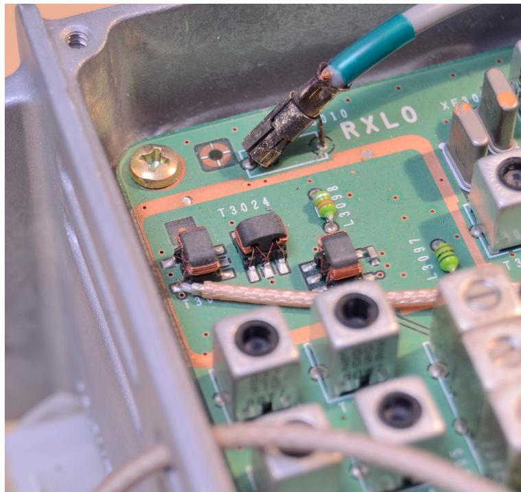
Fig 6 – Connection to T3022 for 2<sup>nd</sup> Rx function
