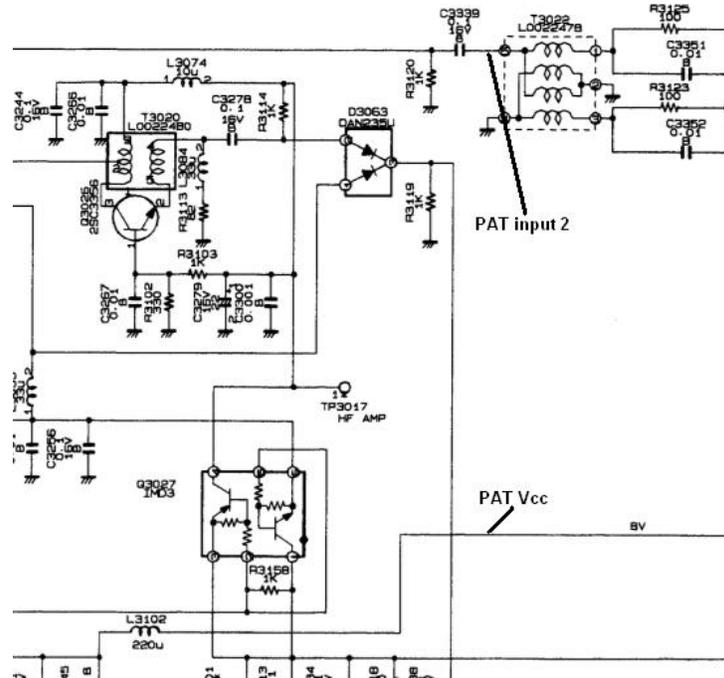
Fig 5 – PAT input for 2<sup>nd</sup> Rx function – other connections also shown
