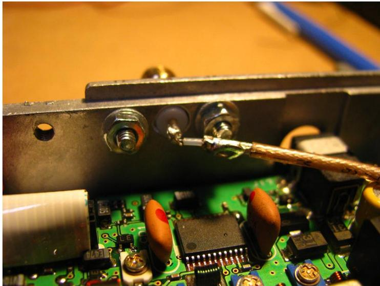
**Fig 7 – Correct method of termination for the RG178 cable**
