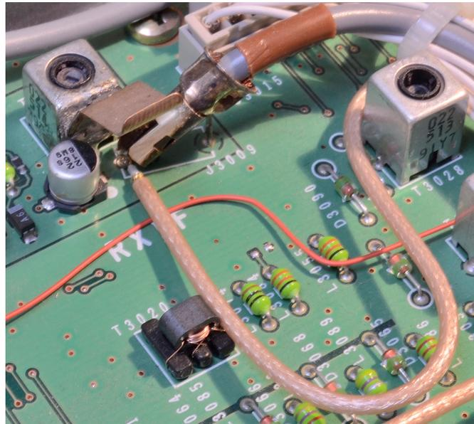
Fig 3 – Coax connection at J3009 for PAT
