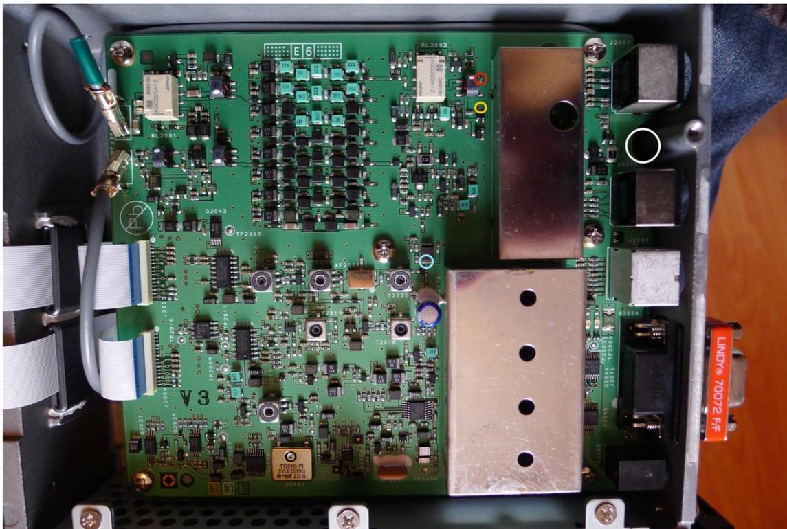
Fig 1 – View of PAT inside FT450, showing connection points. The light blue circle shows the IF Tap point, the red circle shows the 2<sup>nd</sup> Rx tap point and the yellow circle shows where RxB can be found. The white circle shows where the output coax leads down to the SMA output connector.
