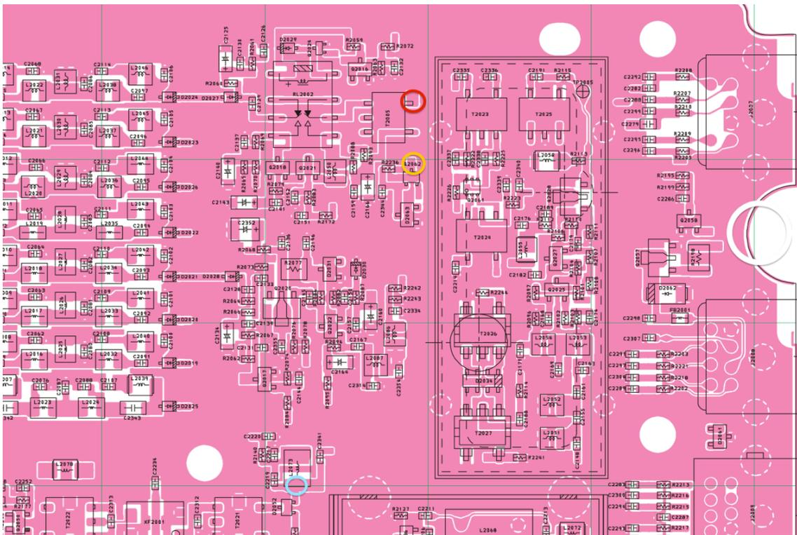
Fig 2 – Part view of the FT450 PCB overlay showing the connection points for the PAT input (light blue circle), and RxB (yellow circle)
