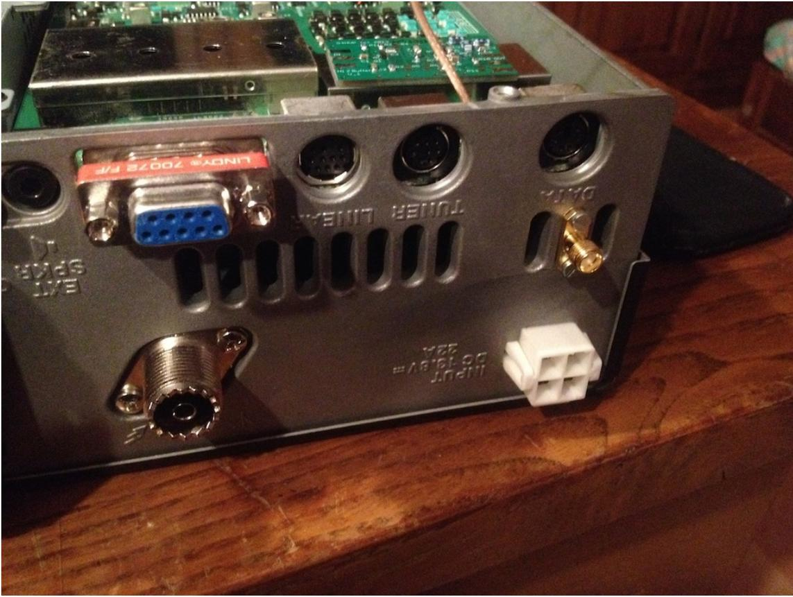
Fig 4 – View of rear panel with SMA connector in place
