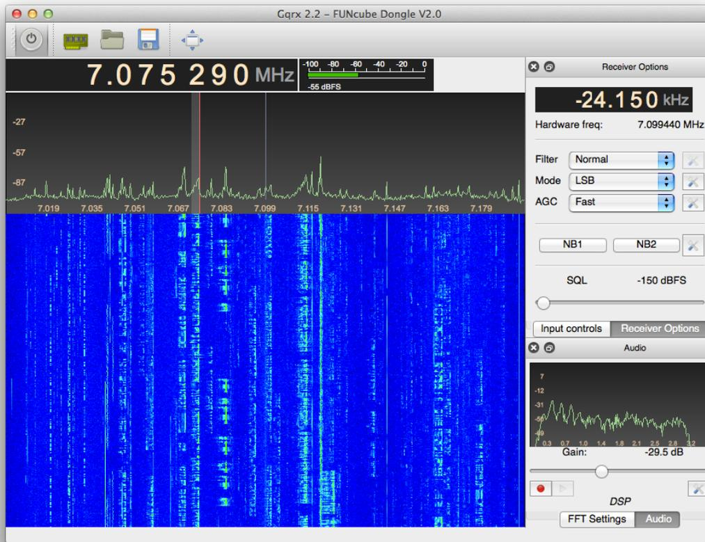
Fig 7 – Sample output of FT450 via PAT, using Funcube Dongle Pro Plus and GQRX
