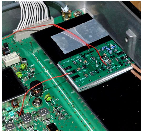
Fig 2 – General view of PAT inside FT950
