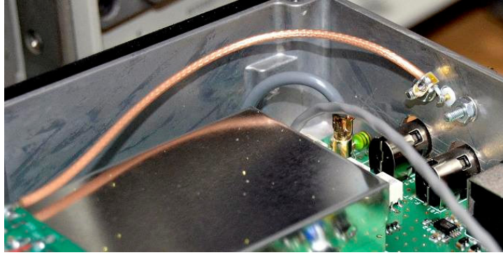
Fig 7 – Routing and termination for the RG178 cable
