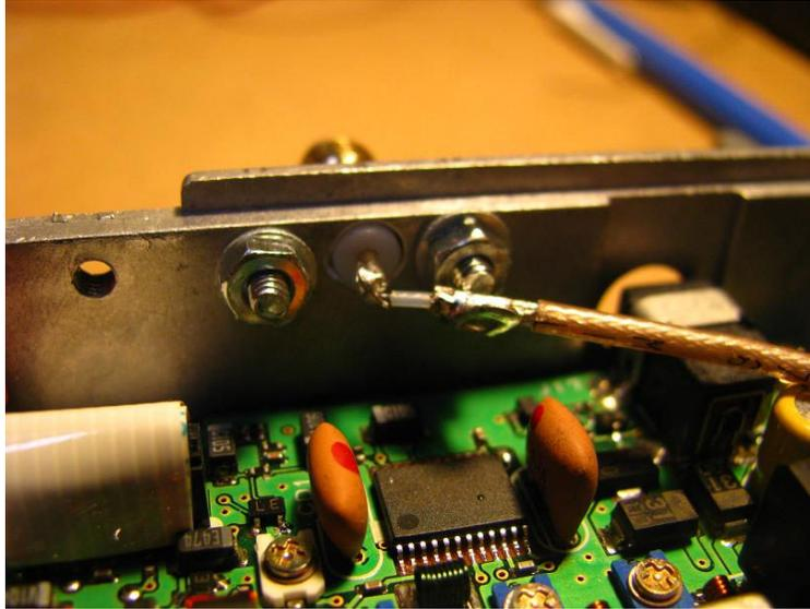
**Fig 9 – Correct method of termination for the RG178 cable**
